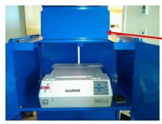
Using the barrel key, open the front of the Auto**MARK** cart.
