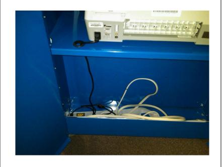
Feed the cord through the opening in the cart and plug into the outlet; use extension cord if necessary.
