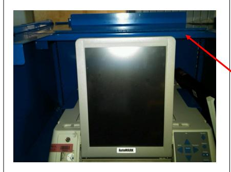
Lift lid as high as it will go and carefully pull the monitor up and out
