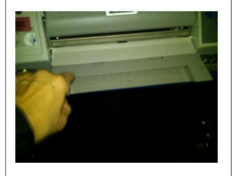
Lift the ballot feed tray up and out to accept ballots for marking
