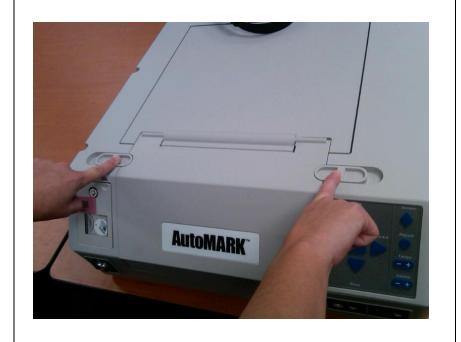
Slide the plastic clips towards the outer edges to release the top cover of the machine.
